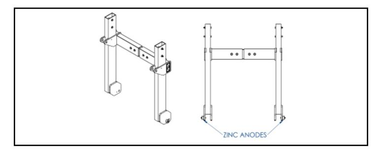
Main beams each get two zinc anodes. 4 cylinder beams get one on each lower cylinder mount. 2 cylinder beams get both anodes on one lower cylinder mount.
